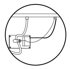
• Ensure the black wire from the system is connected to the igniter.
